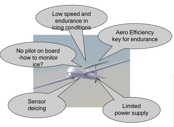
Development and miniaturization of ice sensor • System design and how to use the ice sensor to achieve low power consumption
